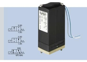
Direct acting medium separated 2/2- and 3/2-way Rocker Solenoid Valve for control of aggressive fluids and gases in analytical medical applications, the food industry, and also the chemical industry for dosing, filling, mixing and distribution.
