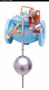
The Apollo Series A800 Float Control Valves are designed to maintain a desired level in a tank or reservoir by opening for filling the tank when fluid is below the high level point and closing tightly when the desired level is reached.
