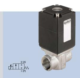
The direct-acting solenoid control valve, Type 2875, (49 mm installation width) is used as the regulating unit in control loops. Due to an elastomeric seat seal the valve closes tight, up to the DN specific nominal pressure.
