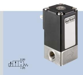
The direct-acting solenoid control valve, Type 2873 ,(32 mm installation width) is used as the regulating unit in control loops. Due to an elastomeric seat seal the valve closes tight, up to the DN specific nominal pressure.
