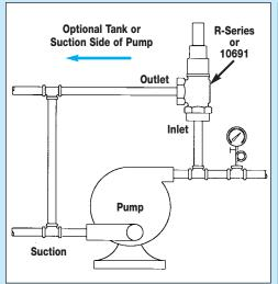
A Relief Valve allows water to recirculate through the pump even when the discharge valve on the pump is completely closed. As a rule, a minimum of 20% of the pump capacity must recirculate to prevent overheating of the pumped liquid.
