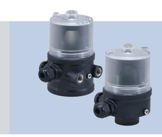
The 8697 pneumatic control unit is optimised for integrated mounting on the ELEMENT 21XX process valve and CLASSIC 20xx series. Mechanical or inductive limit switches register the position of the valve. The integrated pilot valve controls single-acting actuators.
