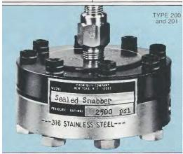
This economical sealed system snubber is ideally suited to applications involving the separation of the pressure instrument system from the pressure actuating material, where cleaning or purging of the lower chamber is not of importance.
