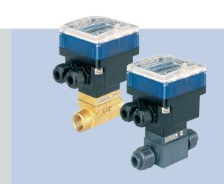
The 8035 batch controller is specially designed for use in neutral, slightly aggressive, solid-free liquids. The batch controller is made up of a compact fitting with paddle-wheel (S030) and an electronic module (SE35) quickly and easily connected together by a Quarter-Turn.
