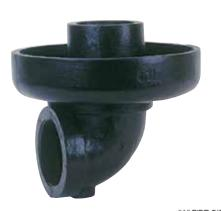
The use of an Apollo International<sup>™</sup> drip pan elbow is highly recommended for steam safety valve installations. The drip pan elbow connects to the valve outlet to safely direct steam discharge away from the valve and into the discharge piping. Condensate is directed to drain. Drip pans offer ideal flow characteristics, and serve to isolate the valve from piping stresses that can adversely effect safety valve performance and longevity.
