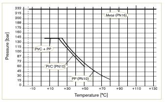
Note: Always take lowest max. medium temp. of both adapter and chosen ELEMENT transmitter.
