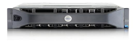
Our Network Video Recorders (NVRs) have Avigilon Control Center preloaded and configured for maximum performance and reliability, making them easy to integrate into any Avigilon surveillance system. NVR servers can record up to 32 MB/s of image data from up to 128 cameras.
