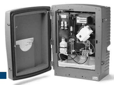
The Hach AMTAX sc Ammonia Analyzer measures NH<sub>4</sub>-N concentrations as low as 0.02 mg/L and as high as 1000 mg/L. With a fast, 5-minute response time, it enhances control of the nutrient removal process. This is no "black box" system—you get transparent, high-quality measurements for reliable values.
