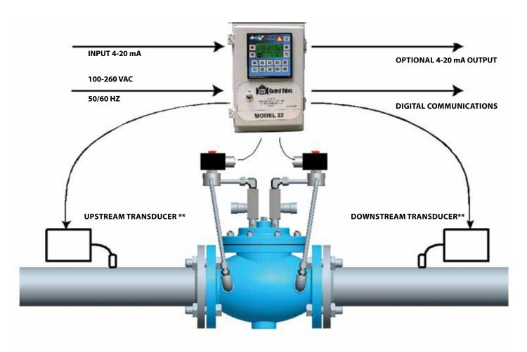
\*\* PRESSURE TRANSDUCER, FLOW METER, LEVEL TRANSMITTER, THERMOCOUPLE OR RTD
