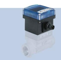
The 8032 flowmeter consists of a SE32 transmitter and a S030 fitting. It is used for measuring clean, neutral or aggressive liquids. It is available with freely configurable switching outputs (transistor or relay) or 4-20 mA process output value.
