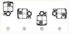
If the absence of any air bubbles cannot be guaranteed, the device should be fitted on a horizontal pipe, with the electronic enclosure facing down. This way, the bubbles will not interfere with the circulation of ultrasound waves.
