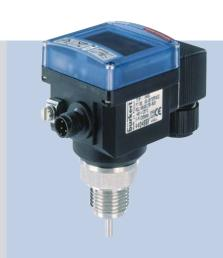
This intelligent sensor / switch with a particularly large display is designed specifically for monitoring limit values or an on/off or continuous control loop. The switching points can be programmed directly via buttons on the display or optionally externally by a PLC via a 4-20 mA standard signal input. In addition, the process value can be transmitted via a 4-20 mA signal to the PLC.
