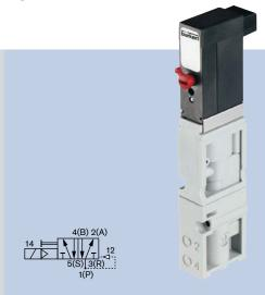
A compact manifold with a pitch of 11 mm per station can be put together from the components of Type 6525. Type 6525 consist of a pilot flipper valve, Type 6144 and a pneumatic seat valve. The flipper principle allows switching of high pressures together with low power consumption and fast response times. All valves are equipped with manual override as a standard.
