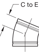
FIGURES 212, 312, & 512 FABRICATED 22½° ELBOW (SEGMENT WELDED)
