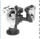
Combination Air Valves consist of Air and Vacuum Valves and a Pressure Valve mounted in a single body, providing the integrity of a single body casting while permitting each valve of the combination to operate as a separate unit. <u>SIZES: 1/2 THRU 24"</u> Cast iron body; bronze and stainless steel trim.
