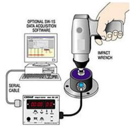
direction and also indicate the number of blows for a selected time period from 0.1 to 9.9 seconds. These instruments have an accuracy of  $\pm 0.5\%$ ,  $\pm 1$  LSD and lbf-in/lbf-ft, kgf-cm/kgf-m, or N-cm/N-m units are selectable. RS-232C output, auto zero reset, auto shutoff and low battery indicator complete the set of features. It is powered by an internal NiCad battery or the included AC adapter.
