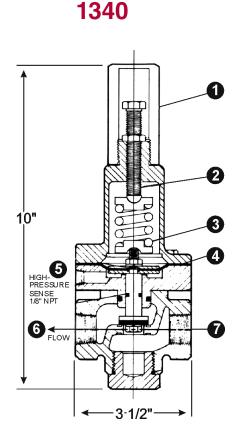
Pilot Materials Bronze B-62 Stainless Steel ASTM A743/CF8M
