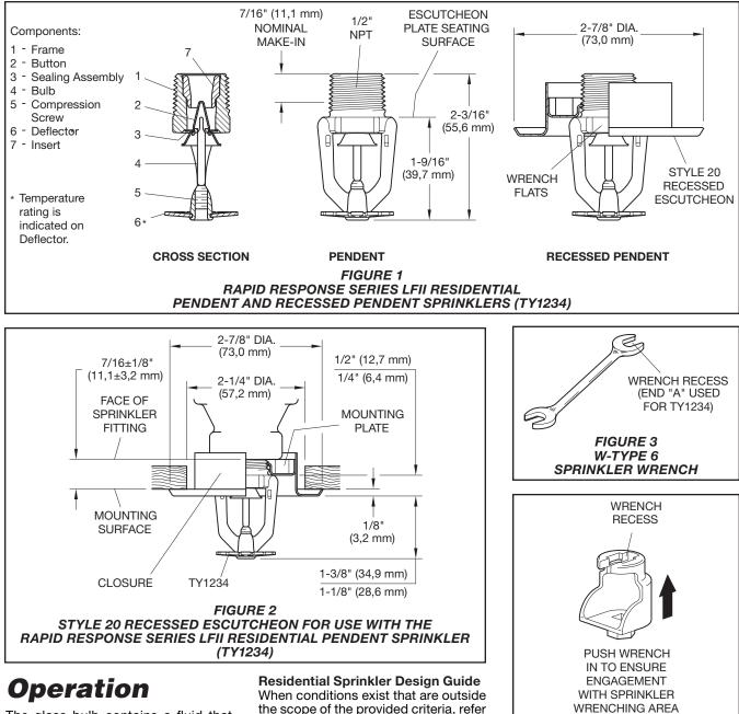
The glass bulb contains a fluid that expands when exposed to heat. When the rated temperature is reached, the
