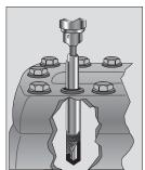
FIRST – Drill a small hole clear through the broken end using a snug fitting RIDGID Drill Guide for precision centering. This centering hole is for the larger drill to follow.
