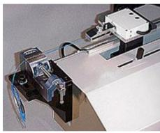
The IMADA Fiber Pull Tester is specially designed to perform pull tests on delicate optical fibers in the manufacturing environment that requires ruggedness and simple operation.
