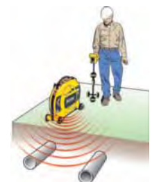
Induce a signal to locate utilities.
