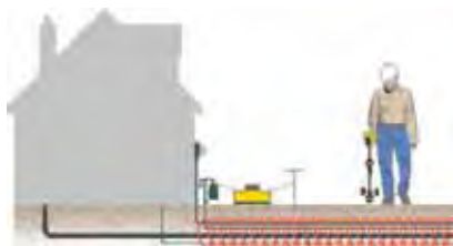
Direct connect to utility lines.
