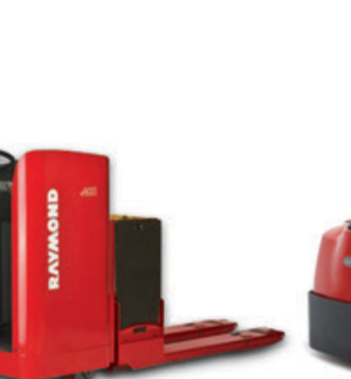
8900 RIDER PALLET TRUCK + Longer travel distances + Heavy duty cycles + Dock, horizontal transport and order picking + Load Capacity lbs. (kg): 6000, 8000 (2722, 3629)
