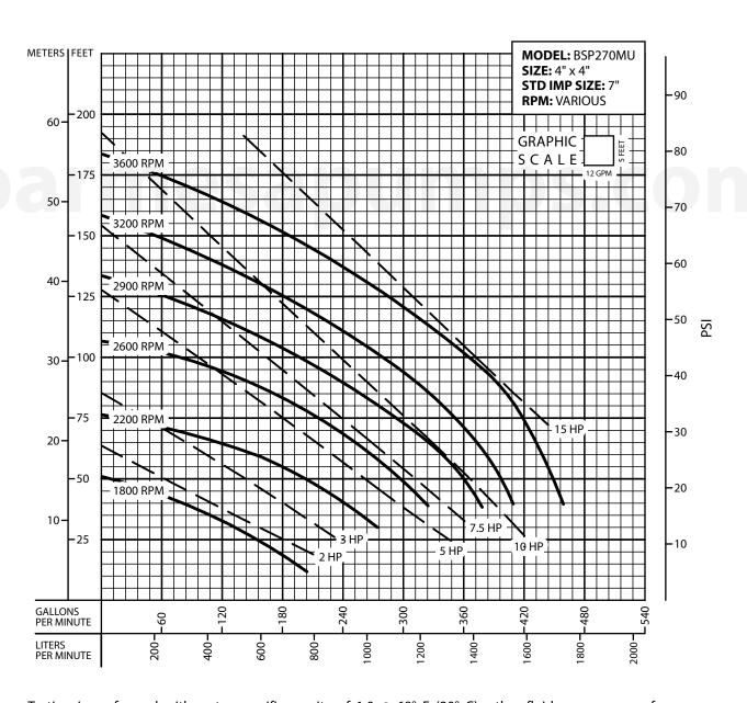
Testing is performed with water specific gravity of 1.0 @ 68° F (20° C); other fluids may vary performance.
