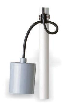
This pump switch is designed to directly control pumps up to 3/4 HP at 120 VAC and 2 HP at 230 VAC in non-potable water and sewage applications. The switch is not sensitive to turbulence, allowing it to be used in both calm and turbulent applications.
