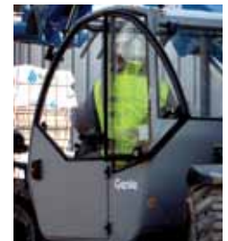
Door with 2 sections: steel on bottom, glass on top. Both sections open separately
