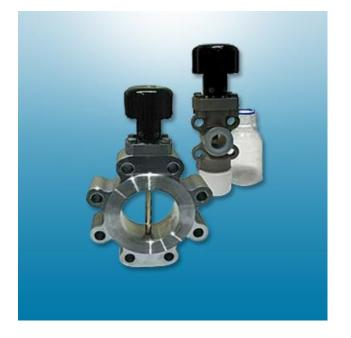
The BTSV-SB series in-line closed-loop sample valve system is engineered to effectively collect representative sample of hazardous process media. The dead space free design can be installed in both horizontal and vertical piping thus allowing the media to constantly flow through the valve and around the conical spindle. Sample bottles either open top or sealed with septums can be directly attached beneath the valve to facilitate the sampling process.
