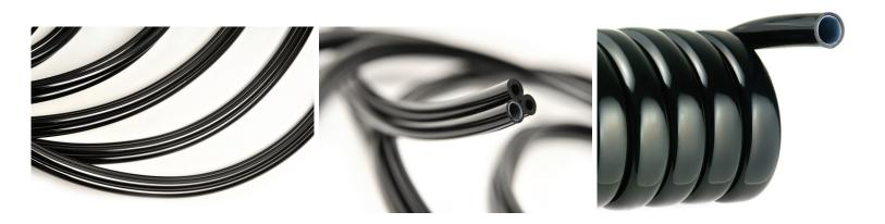
**Envir-A-Line XX** composite tubing is commonly used for the conveyance of a wide variety of **gases**, including **refrigerants** and **hydrocarbons**. It has a unique **co-extruded** construction, incorporating a highly inert **Hytrel**® liner that exhibits excellent dielectric properties as well as superior barrier performance to nonpolar materials, even at elevated temperatures. Because Hytrel® has no plasticizers it does not outgas.
