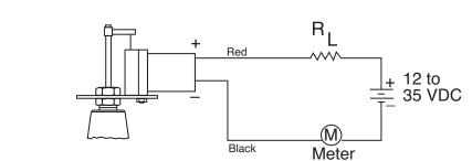
Coupler gap is set with valve in fully closed position. This establishes the minimum mechanical position for 4 mA output.
