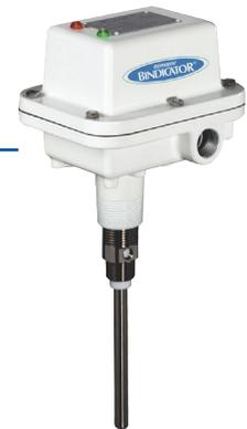
Flo-Guard™ provides reliable detection of leaks, broken bags and filter failures in powder and bulk solid applications. Flo-Guard detects the flow of dust and granular materials by using a floating reference point and a digital triboelectric microcontroller. This technique of measuring the flow of dry materials eliminates instability common in other flow switches.
