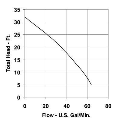
Chem-Resist Type/U6K-E (manual) ES (automatic) -.75HP Voltage 115 or 220 Volt Model – Chem U6K-D (manual) DS (automatic) Voltage 230 or 460 Volt
