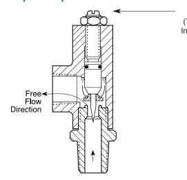
**Free Flow**, is against the direction of the needle. The disc is forced off its seat by line pressure allowing full capacity flow through the control
