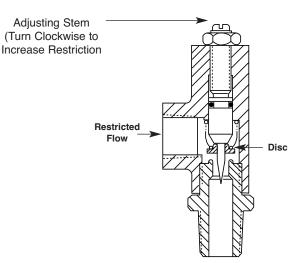
**Restricted Flow**, is in the direction of the needle. This disc is forced against its seat by line pressure. Flow is metered through the control by the fine taper of the needle and the small openings in the disc.
