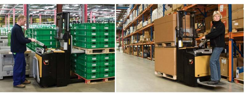
Designed for efficient pallet transport, the **NPV20ND** allows two pallets to be moved simultaneously. This makes it ideal for the loading and unloading of lorries as it has the ability to stack two layers of pallets on top of each other.
