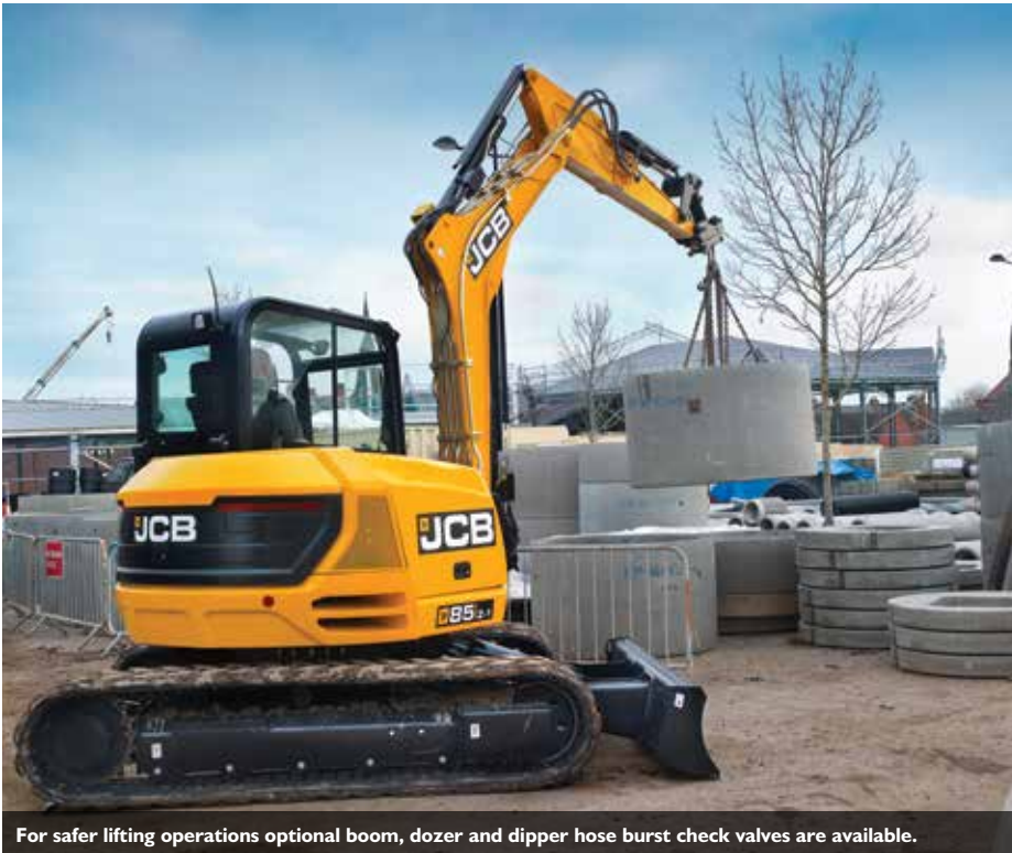
The heavy-duty boom cylinder guard provides excellent protection when loading.
