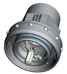
The pressure balanced design of the Cla-Val Model 346GF Emergency Breakaway Coupling incorporates a number of springs and o-rings that limit fuel leakage. The main swivel o-ring, which is located on the Inlet Half can be easily changed with the Coupling is disconnected. This o-ring can be changed on the flight line.
