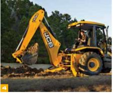
Rear stabilizers are equipped with twin hose burst check valves (HBCVs), which means the legs can't move during machine operation.
