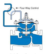
**Full Open Operation** When operating pressure below the diaphragm is applied and pressure is relieved from the cover chamber, the valve is held open allowing full flow.
