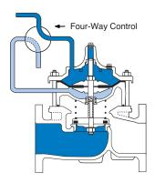
**Tight Closing Operation** When pressure below the diaphragm is relieved and operating pressure is applied to the cover chamber, the valve closes drip-tight.
