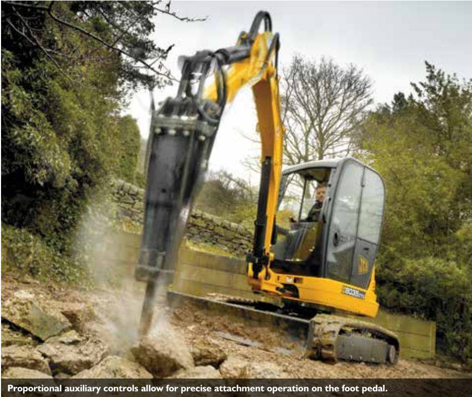
Proportional auxiliary controls allow for precise attachment operation on the foot pedal.
