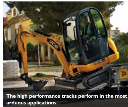
New dig-end geometry provides extra reach, load-over height, and dig depth.
