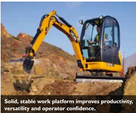
New dig-end geometry provides extra reach, load-over height, and dig depth.
