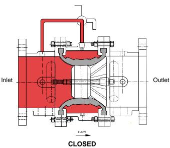
Water pressure (equal to inlet pressure) from valve inlet is applied to the control chamber. Valve closes bubble tight.
