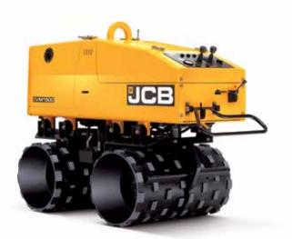
The JCB VM1500 high-impact roller is the best performer of its type in the industry and, as you would expect, it is designed for maximum productivity on a variety of different soils. There are two models available: the manually controlled VM1500M and the remote controlled VM1500F. Both feature 4-drum drive steering and a center mounted vibration exciter system.
