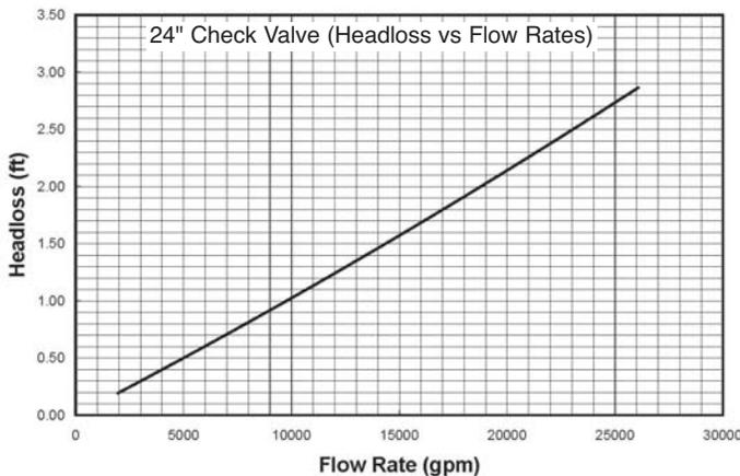
Sample Flow Rate vs Headloss Graphs. Other size charts available upon request. Based on flow testing at Utah State University.
