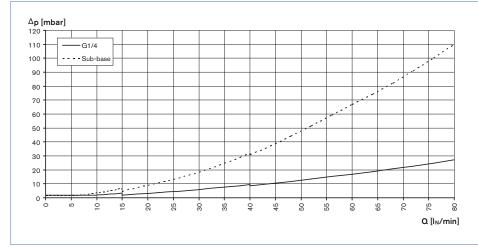
The diagram shows exemplarily the pressure loss characteristics when air flowing through.
