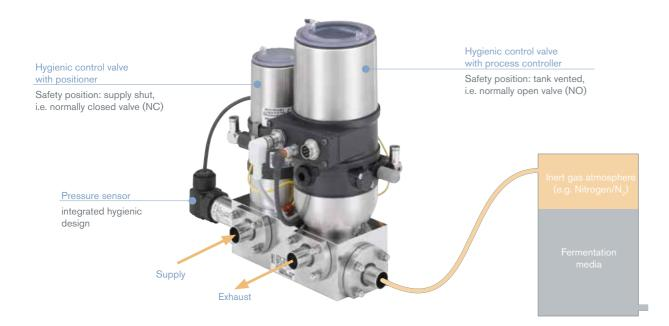
The hygienic control valve system on the left clearly demonstrated its all-time high safety values in tank blanketing. The system itself builds upon two hygienic control valves of Type 2380. These compact, lightweight and CIP/SIP-capable valves are suitable for virtually any pressure, low-flow and filling control application in hygienic environments, where they also introduce new levels of precious productivity and quality.
