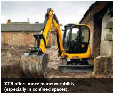
Superb digging and tracking performance via the load-sensed hydraulic system.
