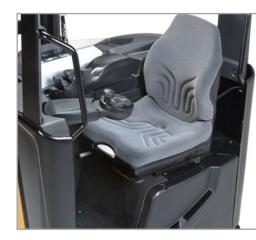
The latest display panel, hydraulic control unit and steering console make operation easy, comfortable and precise. The spacious operator compartment (right) features a fully adjustable seat to meet each individual's needs.
