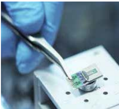
Insertion and bonding of chips.
