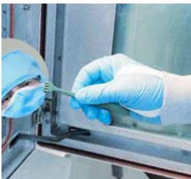
The surfaces are cleaned and activated using a plasma beam.
