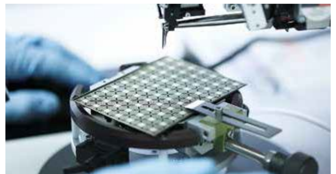
The test piece for the electrical connections is located under the manual bonder for the deep access wedge.
