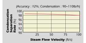
Separation rate (%) is given as: quantity of condensate discharged quantity of incoming condensate
